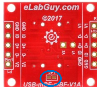
Figure 6: PCB back with optional Jumper connects Shield to GND
